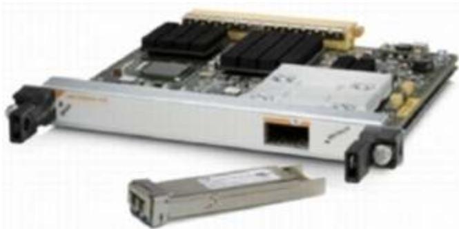
Figure 1. Cisco 1-Port 10-GE SPA with XFP Optics
