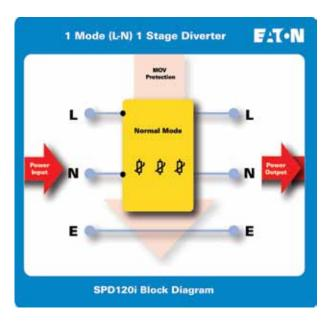
The SPD120I is designed to protect single-phase power systems against surges & spikes caused by lightning strikes & other electrical sources. The unit is intended for point-of-entry or main board protection in medium to high exposed locations. SPD120I are easily configured for L-N or L-E protection for installations adjacent or remote from the M.E.N. link, which means it can provide protection for commercial buildings to rural sites.
