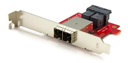
This Mini-SAS adapter lets you convert two internal SFF-8643 ports on a controller card into two external SFF-8644 ports. This enables you to connect external SAS or SATA drives in devices such as a Direct Attached Storage (DAS) device to an internal backplane or SAS controller for additional storage.
